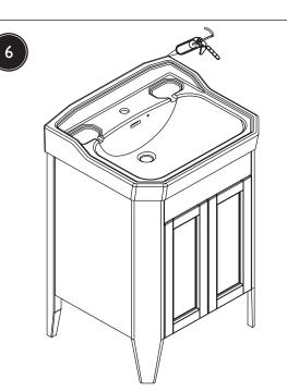
Use silicon sealant where necessary to ensure the basin edges are sealed and water tight to the furniture and wall. Refer to any instructions with handles when fitting to the doors.
