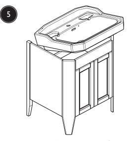
Fix basin to the wall using suitable fixings (not-supplied). To ensure the basin sits correctly on the unit a shim may be required behind the splash back.
