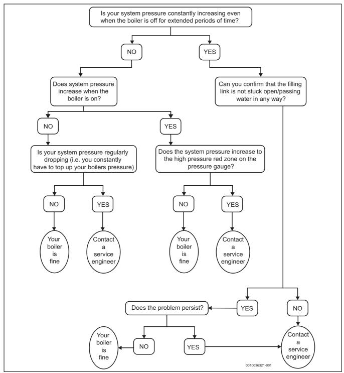
Fig. 8 Gassing flow chart
