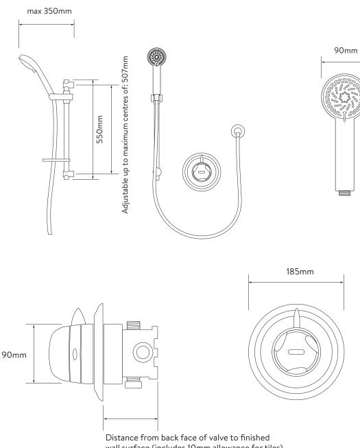
wall surface (includes 10mm allowance for tiles) MIN 60mm, MAX 100mm
