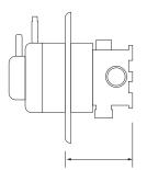
160mm min, 100mm max from back face of valve to finish / tiled wall surface (10mm allowance for tiles)
