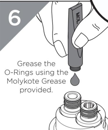
Grease the O-Rings using the Molykote Grease provided.
