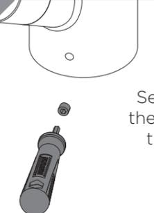
Secure in place with the grub screws using the tool provided.
