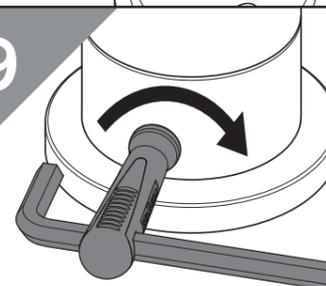
Thread the hexagonal key through the EasyFit tool and tighten the grub screws with an extra 1/2 turn.
