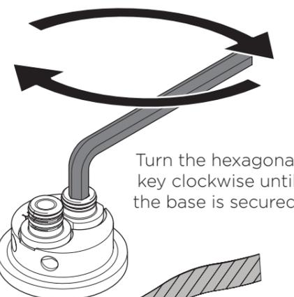
Turn the hexagonal key clockwise until the base is secured.
