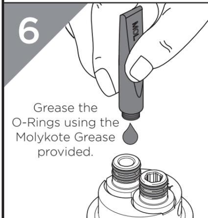
Grease the O-Rings using the Molykote Grease provided.
